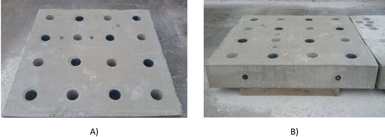
Figure 2.4. PCC Slabs for extracting the cores at the Illinois Center for Transportation (ICT).
